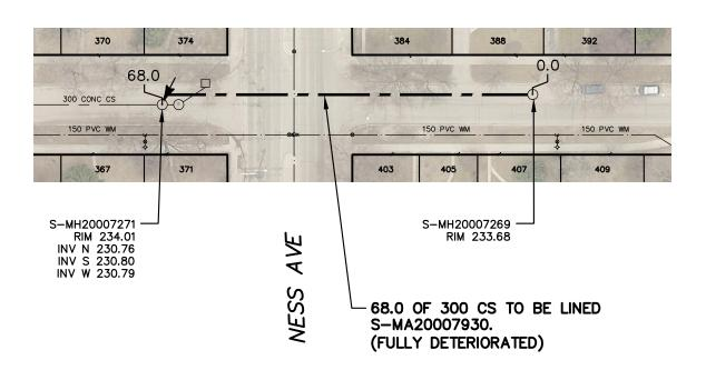
SEWER JUNCTION INFORMATION FROM SEWER VIDEO INSPECTION SEWER ID S-MA20007930 DISTANCE FROM MH ID S-MH20007269 DISTANCE DIAMETER CLOCK 4.0 8.7 150 23.4 150 150 24.4
