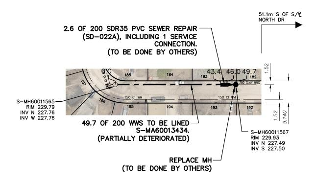
SEWER JUNCTION INFORMATION FROM SEWER VIDEO INSPECTION SEWER ID S-MA60013434 DISTANCE FROM MH ID S-MH60011565 DISTANCE DIAMETER CLOCK 150 7.5 9 9.9 150 150 24.8 27.2 150 9 42.8 150 45.2 150
