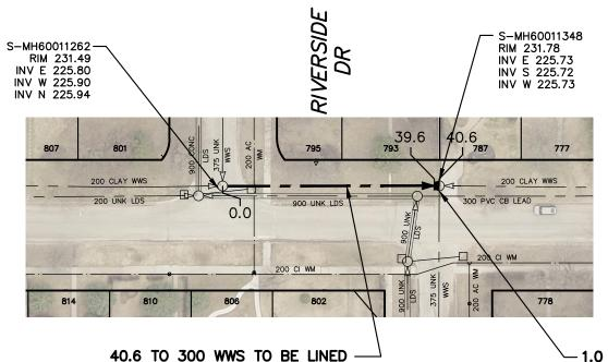
SEWER JUNCTION INFORMATION FROM SEWER ID S-MA60013108 DISTANCE FROM MH ID S-MH60011348 DISTANCE DIAMETER CLOCK
