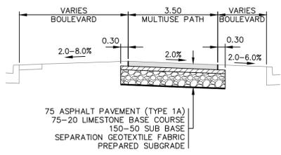
TYPICAL MULTI-USE PATH CROSS SECTION A-A
