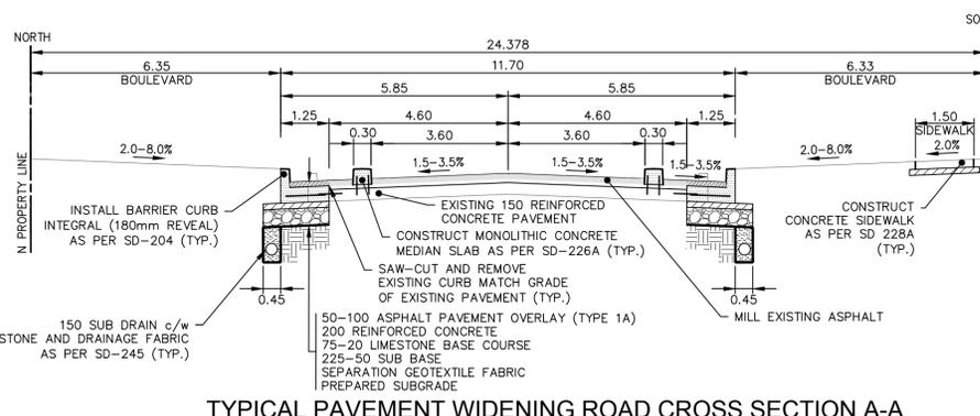
TYPICAL PAVEMENT WIDENING ROAD CROSS SECTION A-A
