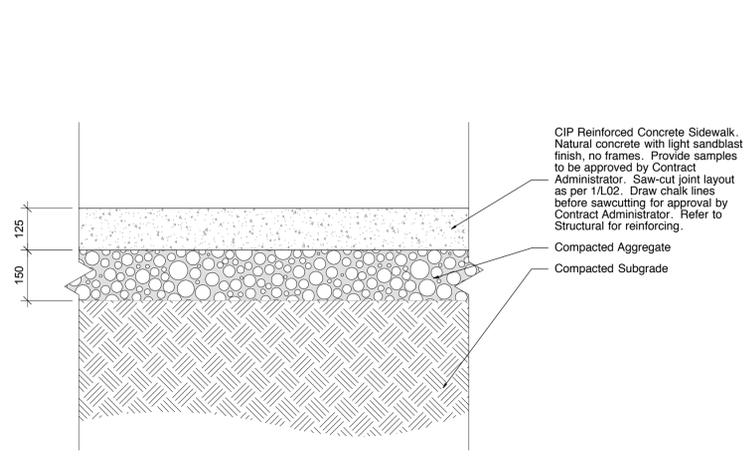
1 C.I.P. Concrete Paving, Typ.
