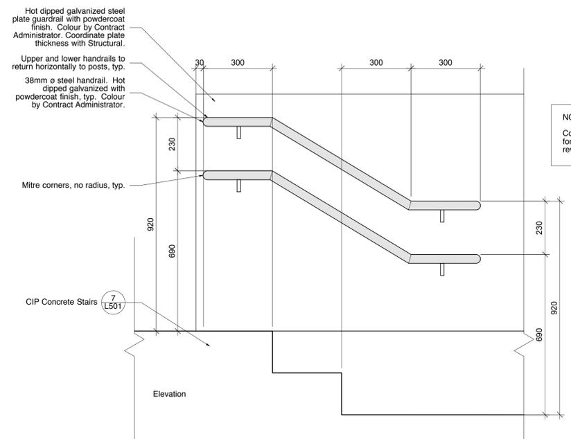
8 Custom Galv. Steel Guard and Handrail at Stairs, typ.
