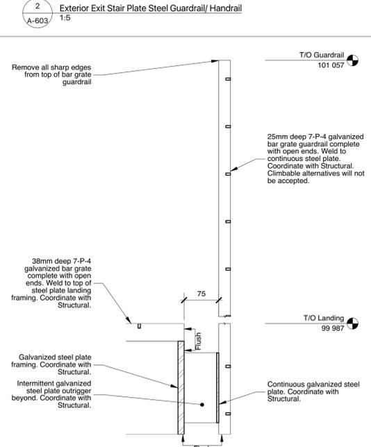
1 Section Detail - Exterior Stair Landing Bar Grate Guardrail
