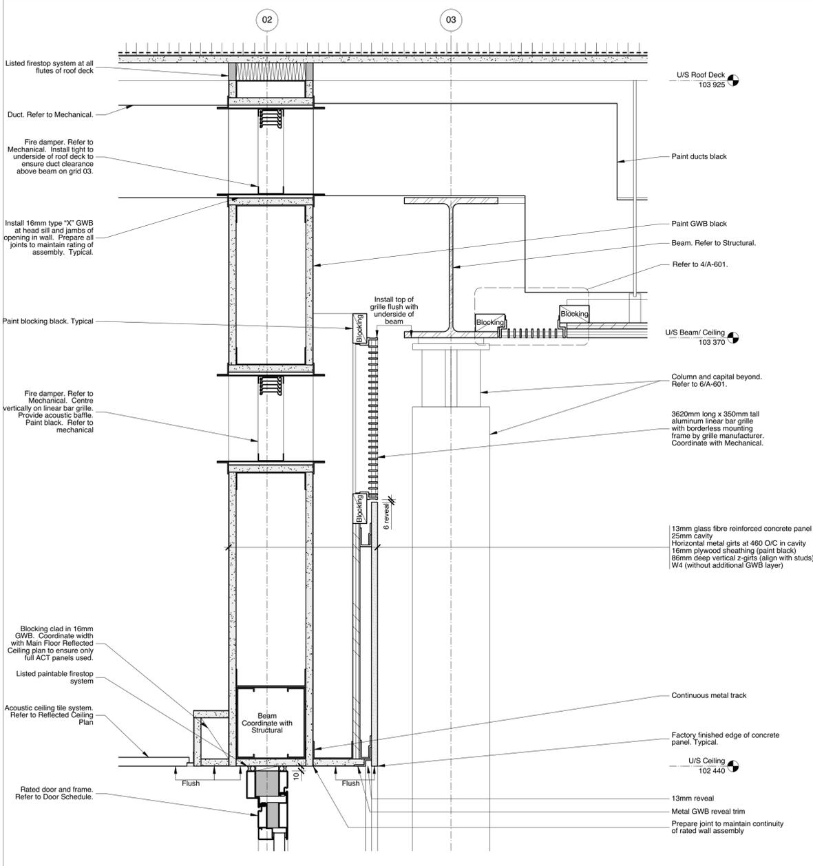
9 Section Detail - Return Air Grille in GWB Ceiling
