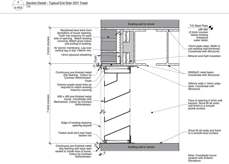
8 Section Detail - Mechanical Louver in Existing Brick Wall
