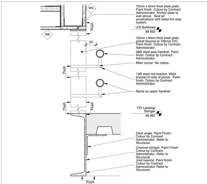
5 Section Detail - Exit Stair 001 Guardrail/Handrail
