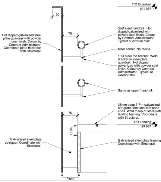
2 Exterior Exit Stair Plate Steel Guardrail Handrail
