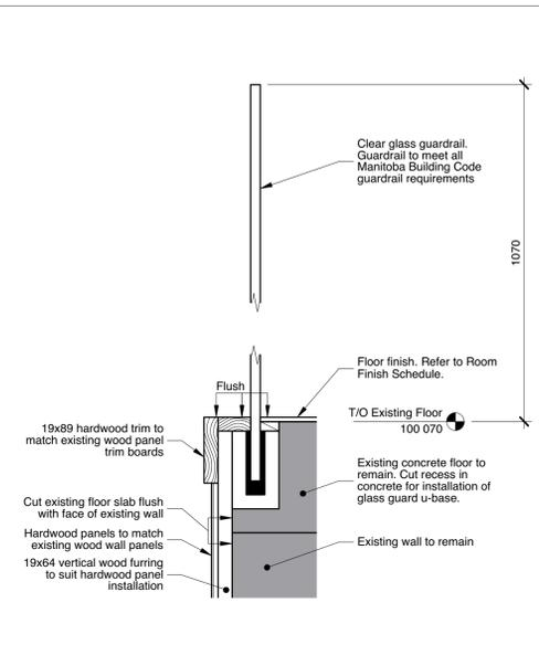
7 Section Detail - Glass Guardrail at Entry Area 100
