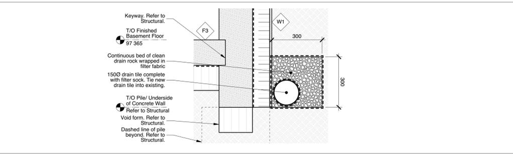
8 Section Detail - Typical Drain Tile
