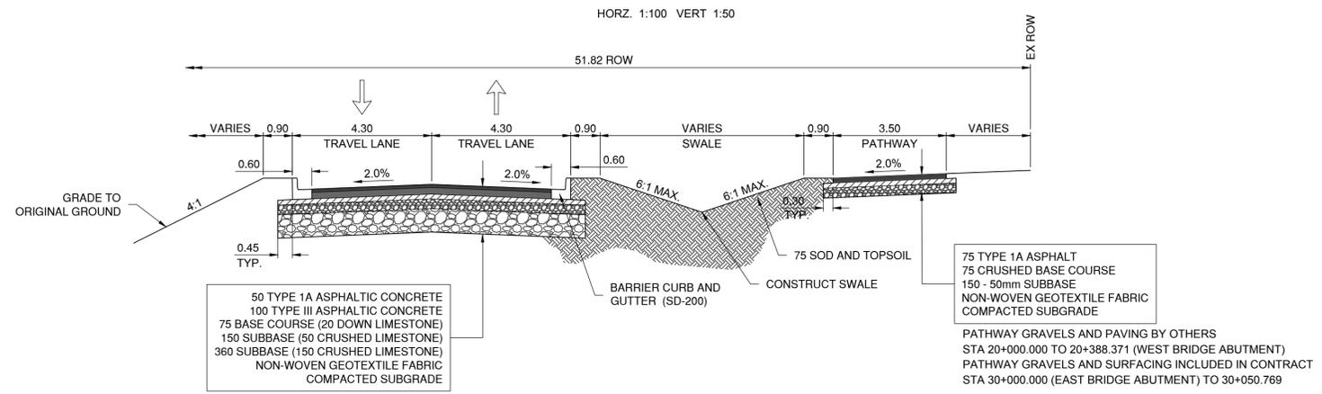
**TYPICAL SECTION - ROAD RECONSTRUCTION WITH PATHWAY/SWALE**
