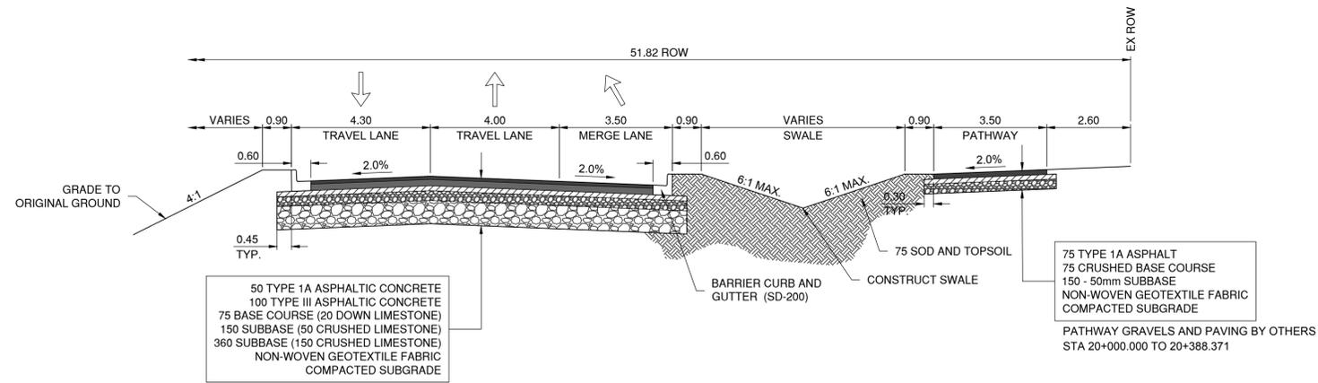
**TYPICAL SECTION - ROAD RECONSTRUCTION WITH AUXILIARY LANE**
