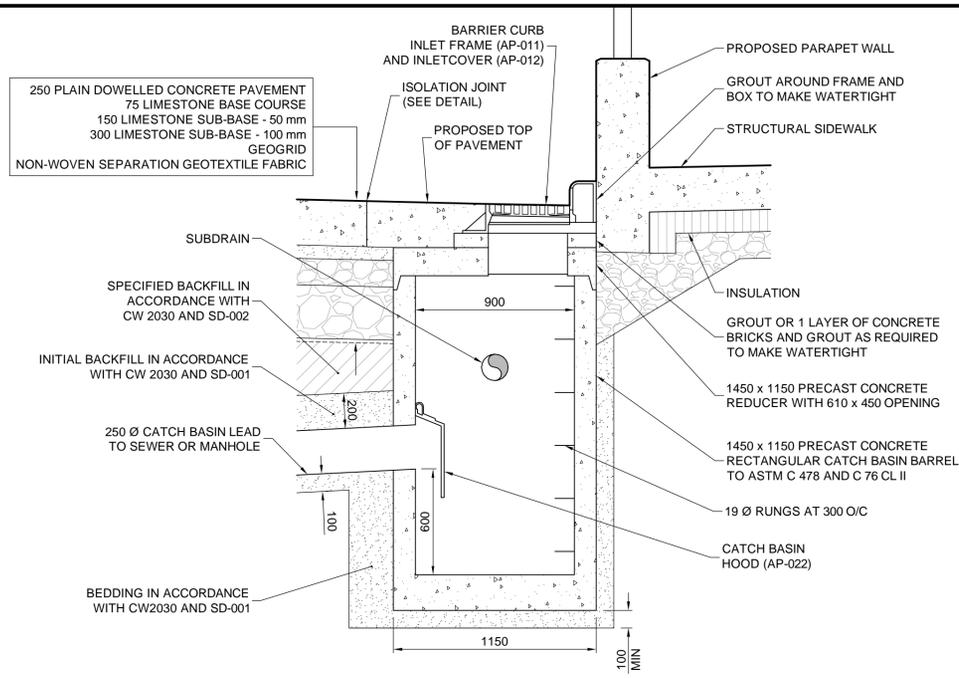
**1 PRECAST RECTANGULAR CATCH BASIN (AT NEW PARAPET WALL)**
