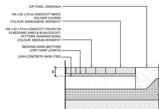
3 UNIT PAVERS IN CONC. BLOCKOUT - SIDEWALK
