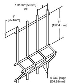
THE ECO FENCE SYSTEM IS AN ASSEMBLY OF TWO PANELS
