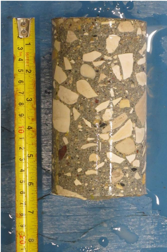
Figure 27 - Core no. A7, west abutment
