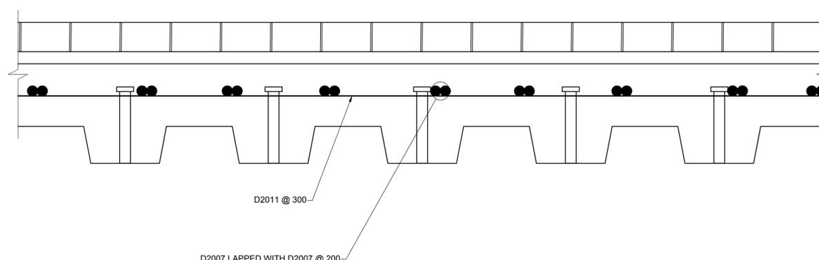
**SECTION - BRIDGE DECK REINFORCEMENT**
