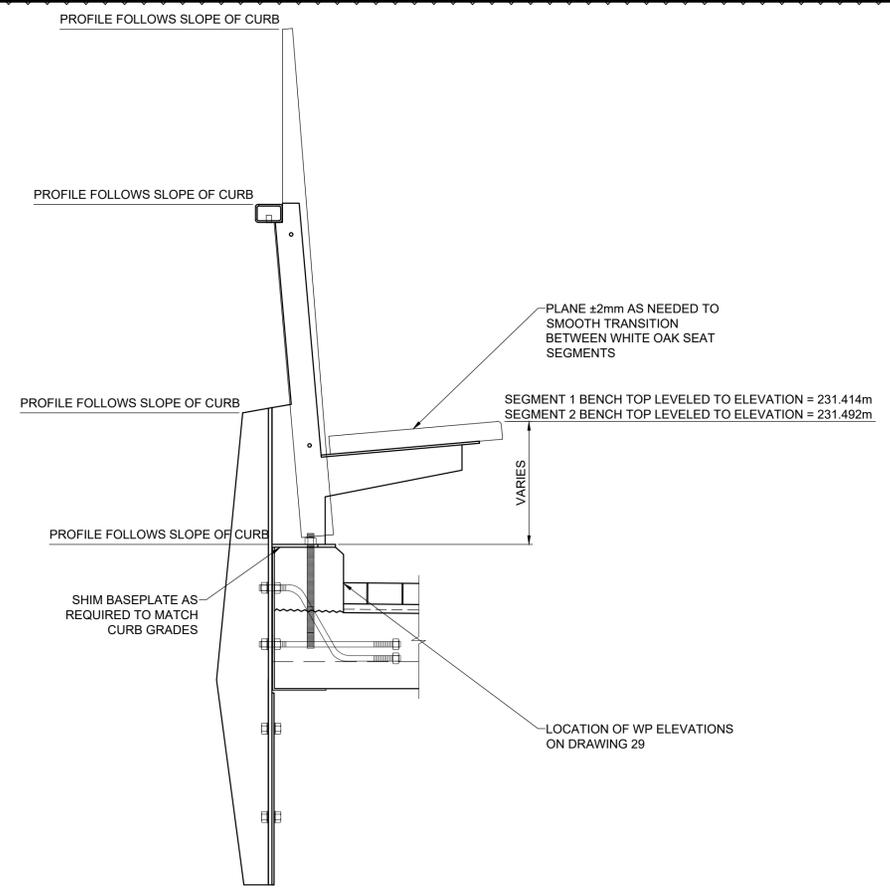
**SECTION - GEOMETRY CONTROL FOR INTEGRATED BENCH**
