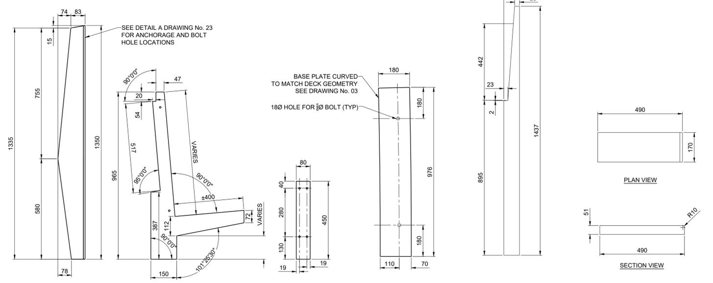
**RAIL POST** SCALE: 1:10    **BENCH PLATE** SCALE: 1:10    **BENCH PLATE** SCALE: 1:10    **BASE PLATE** SCALE: 1:10    **TIMBER POST** SCALE: 1:10    **WHITE OAK BENCH SEAT** SCALE: 1:10
