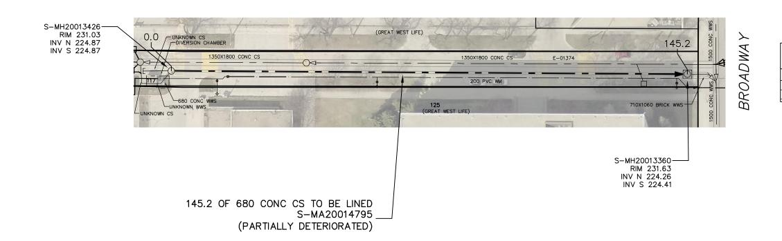
SEWER JUNCTION INFORMATION FROM SEWER VIDEO INSPECTION SEWER ID S-MA20014795 DISTANCE FROM MH ID S-MH00013426 DISTANCE DIAMETER CLOCK \*\*\*\*\* NO SERVICE JUNCTIONS \*\*\*\*
