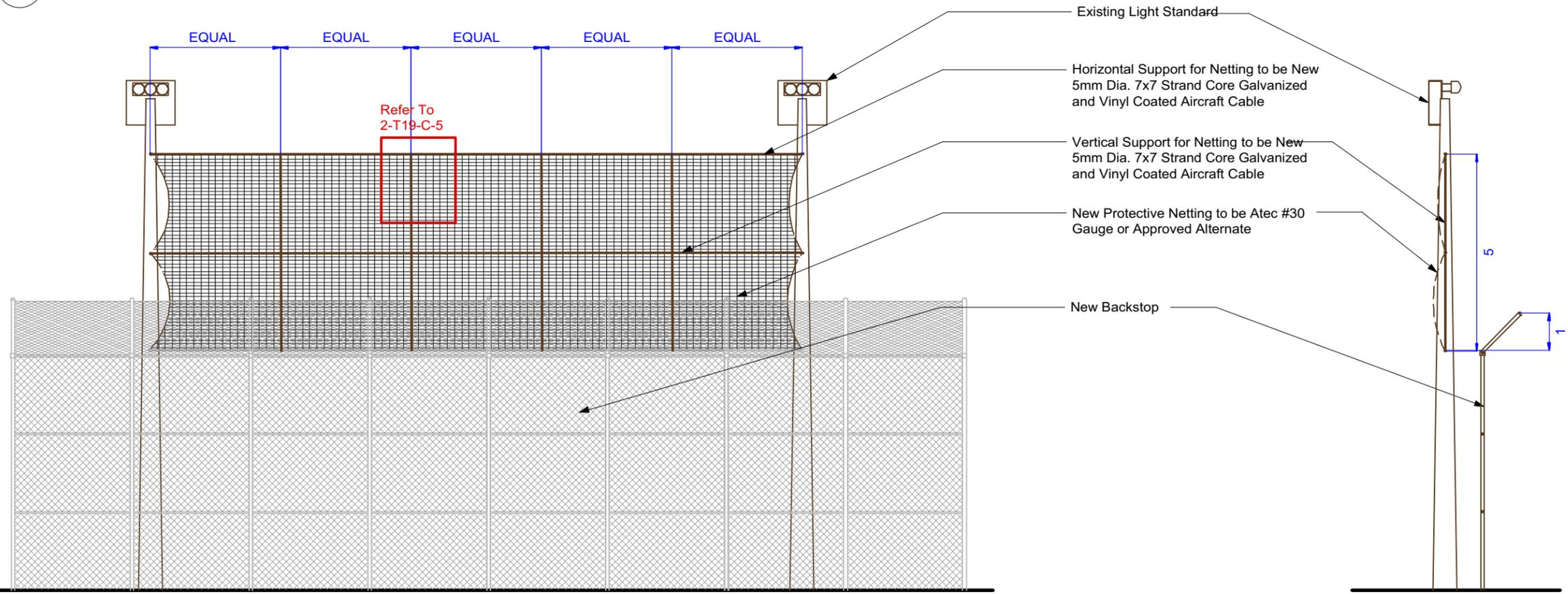
1 PROTECTIVE NETTING AND SUPPORT CABLES (ELEVATION AND SECTION)
