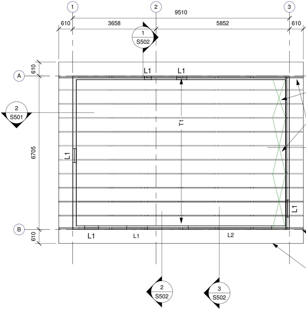
PROVIDE PERMANENT 38x89 VERTICAL CROSS BRACING ON INTERIOR FACE OF TRUSS END WEB AT POLYCARBONATE CLAD WALL. DESIGN OF ADDITIONAL PERMANENT TRUSS BRIDGING OR BRACING BY TRUSS SUPPLIER, REFER TO TRUSS SHOP DRAWINGS AND INSTALL AS PER SUPPLIERS RECOMMENDATIONS.
