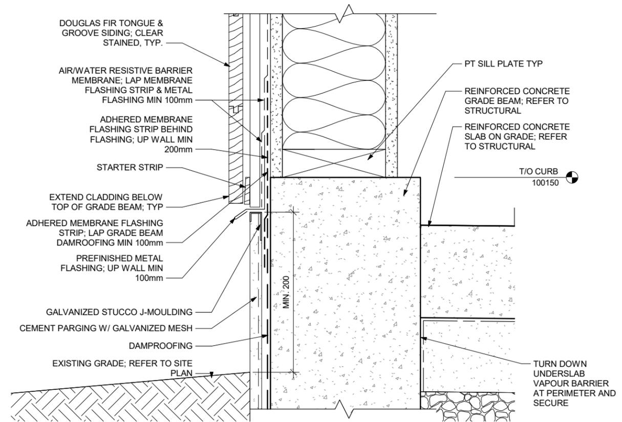
7 SECTION DETAIL - BASE OF WALL - WOOD CLADDING
