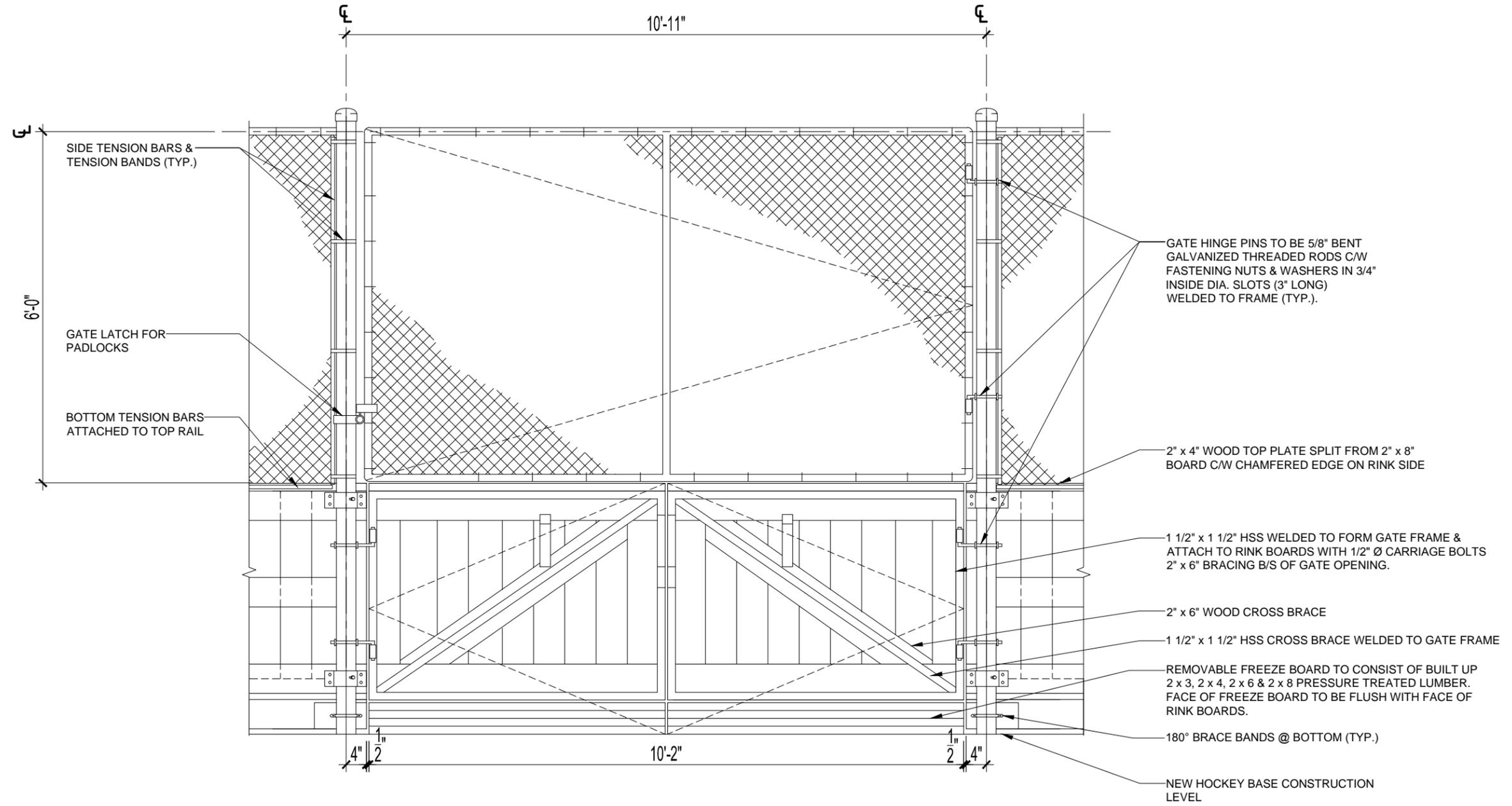
**VEHICLE GATE ELEVATION -SWINGING GATE**
