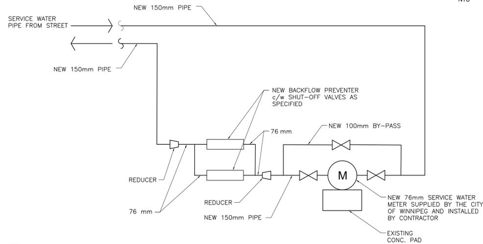
**WATER AND BY-PASS SCHEMATIC DETAIL**
