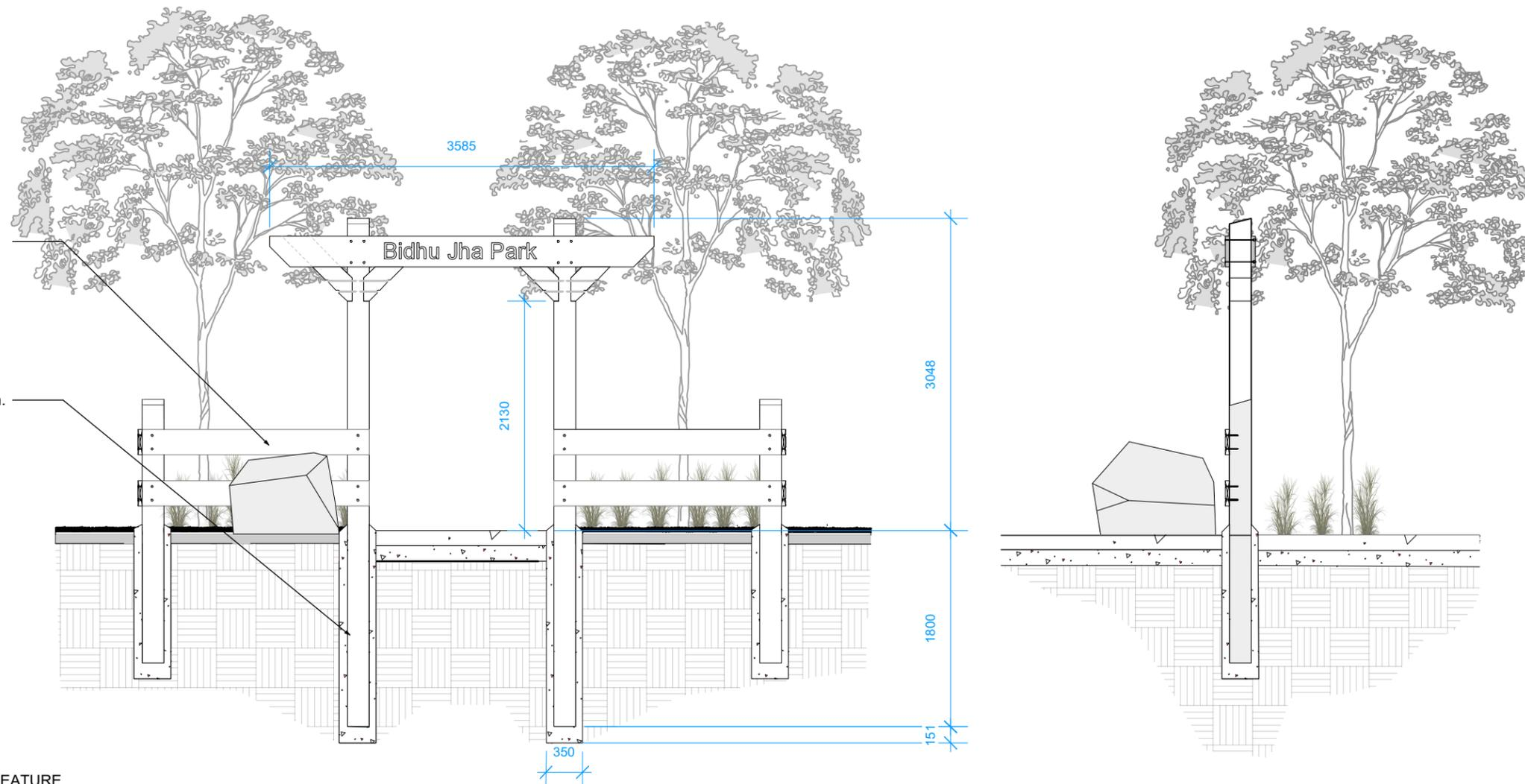
PT Timber fence. Refer to fence detail on M.060-A7
