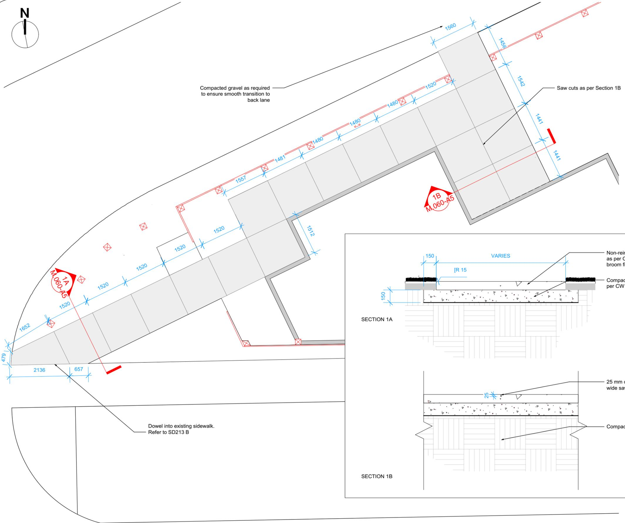
CONTRACTOR TO CONFIRM ALL DIMENSIONS AND REPORT ANY DISCREPANCIES TO CONTRACT ADMINISTRATOR PRIOR TO CONSTRUCTION. LOCATION OF UNDERGROUND STRUCTURES AS SHOWN ARE BASED ON THE BEST INFORMATION AVAILABLE BUT NO GUARANTEE IS GIVEN THAT ALL EXISTING UTILITIES ARE SHOWN OR THAT THE GIVEN LOCATIONS ARE EXACT. CONFIRMATION OF EXISTENCE AND EXACT LOCATION OF ALL SERVICES MUST BE OBTAINED FROM THE INDIVIDUAL UTILITIES BEFORE PROCEEDING WITH CONSTRUCTION.
