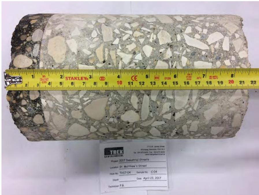
Photo 4: Pavement Core Sample at Test Hole TH17-04
