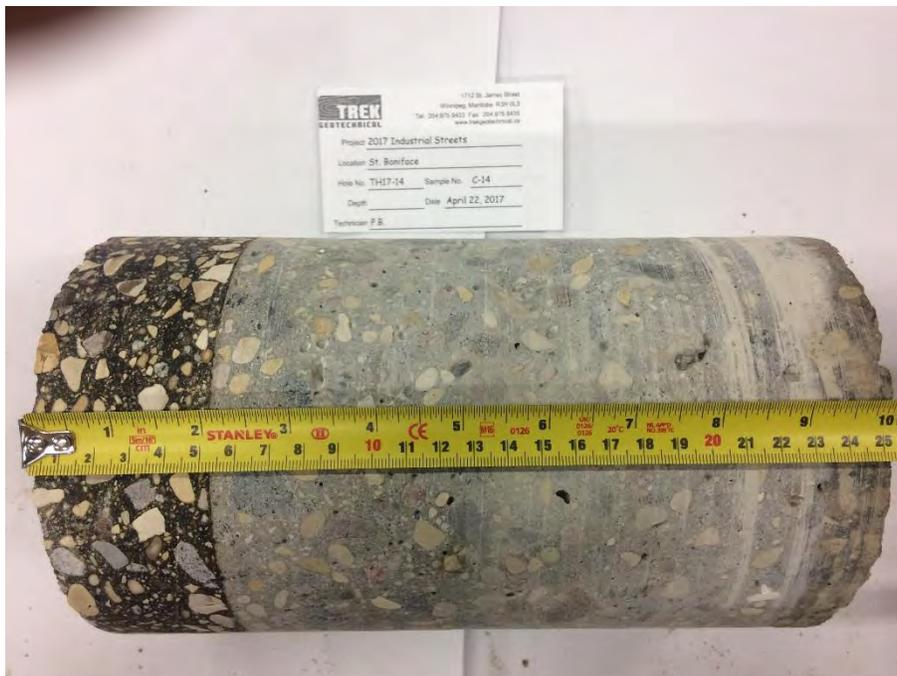
Photo 14: Pavement Core Sample at Test Hole TH17-14
