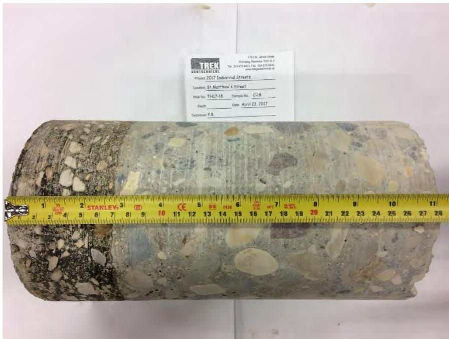
Photo 18: Pavement Core Sample at Test Hole TH17-18
