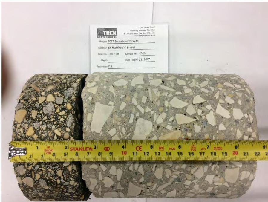
Photo 16: Pavement Core Sample at Test Hole TH17-16
