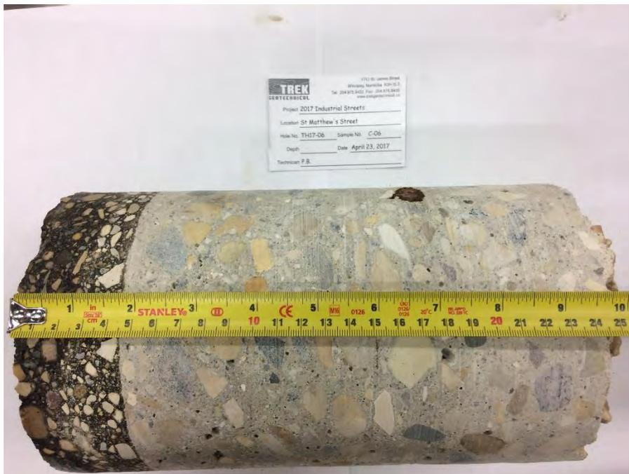
Photo 6: Pavement Core Sample at Test Hole TH17-06
