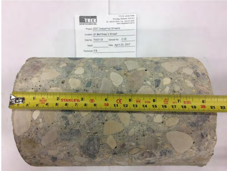
Photo 15: Pavement Core Sample at Test Hole TH17-15
