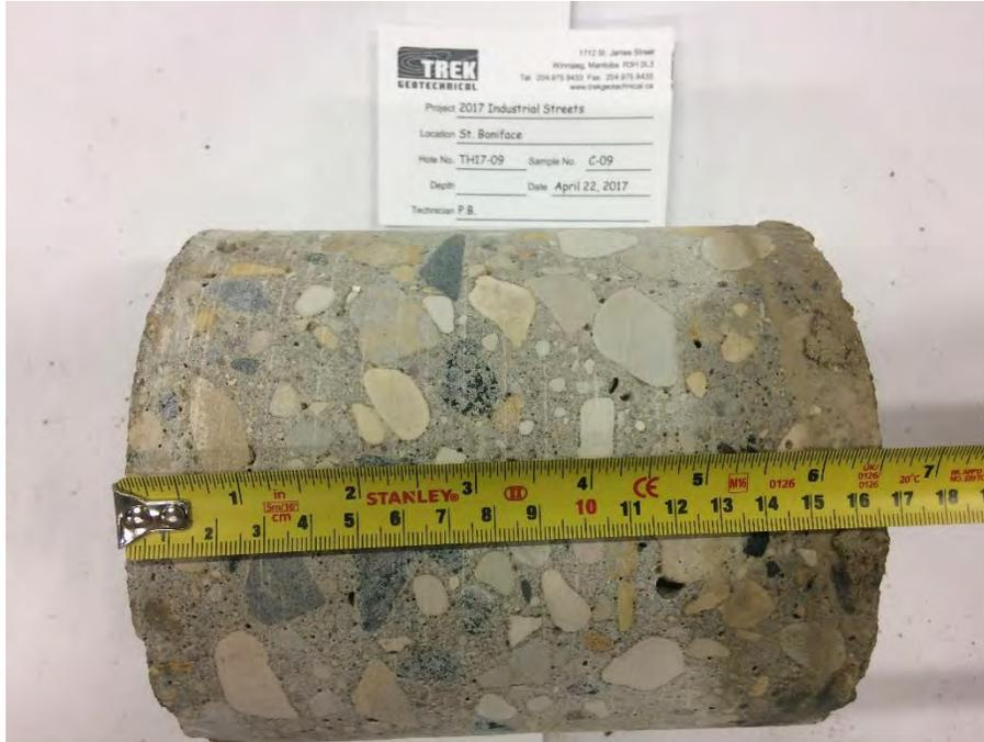
Photo 9: Pavement Core Sample at Test Hole TH17-09
