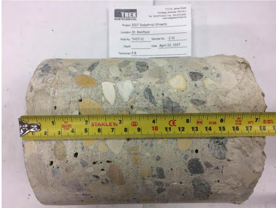
Photo 11: Pavement Core Sample at Test Hole TH17-11
