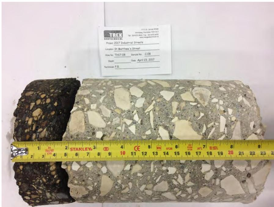
Photo 8: Pavement Core Sample at Test Hole TH17-08
