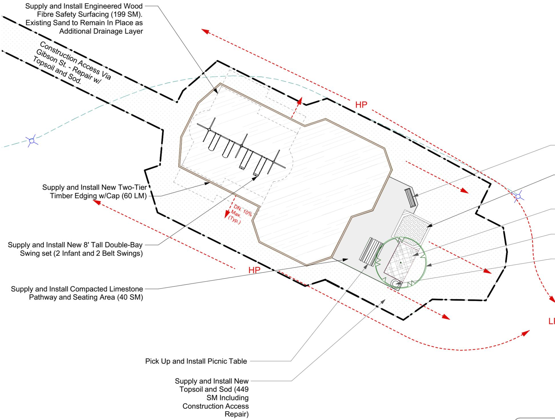
Supply and Install Engineered Wood Fibre Safety Surfacing (199 SM). Existing Sand to Remain In Place as Additional Drainage Layer
