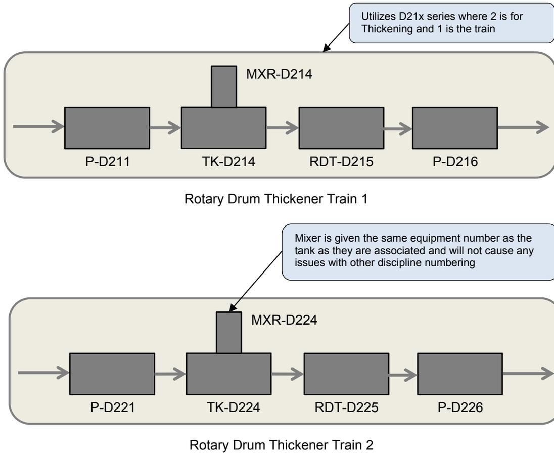
**Figure 2-2 : Sequential Logical Numbering Example**
