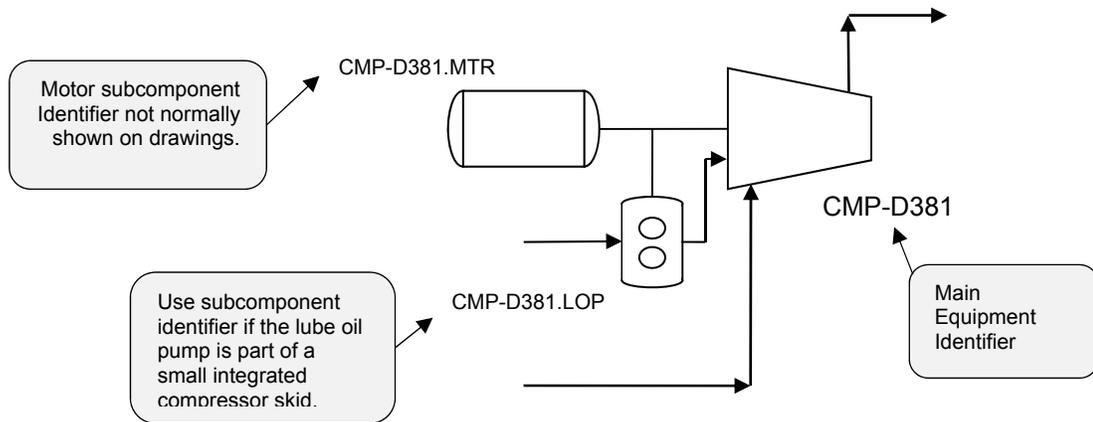
**Figure 2-3 : Lube-Oil Pump Subcomponent Example**
