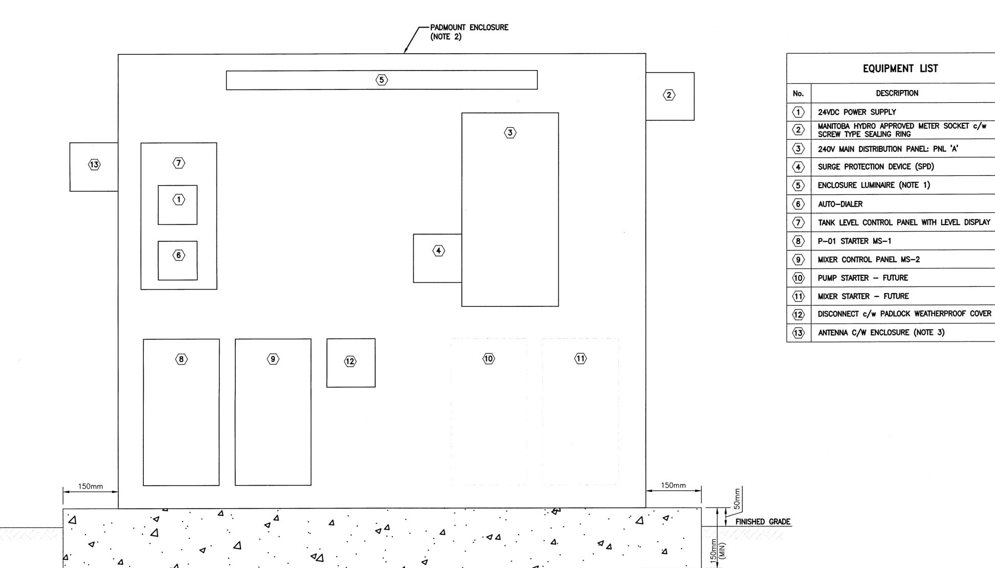
PADMOUNT ENCLOSURE-FRONT ELEVATION SCALE: N.T.S.
