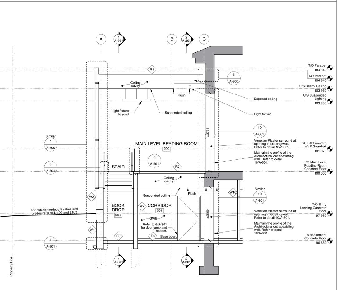
2 North/South Building Section - Main Level Reading Room and Basement Lobby Connection to Existing
