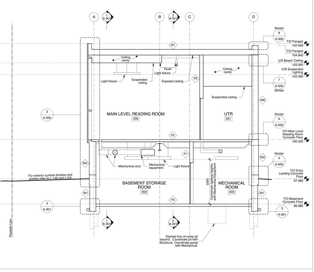
1 North/South Building Section - Main Level Reading Room and UTR
