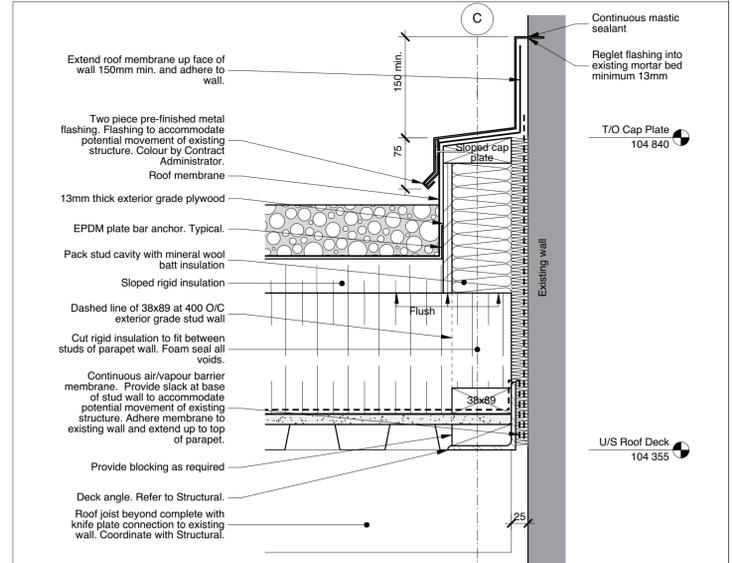
6 Section Detail - Parapet Between Addition Roof and Existing Wall
