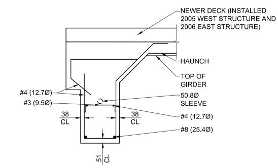
**SECTION - END DIAPHRAGM** SCALE: 1:20
