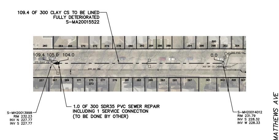
SEWER JUNCTION INFORMATION FROM SEWER ID S-MA20015522 DISTANCE FROM MH ID S-MH20013998 DISTANCE DIAMETER CLOCK 150 10 9.5 \*\*\*\*REVERSAL REQUIRED\*\*\*\*
