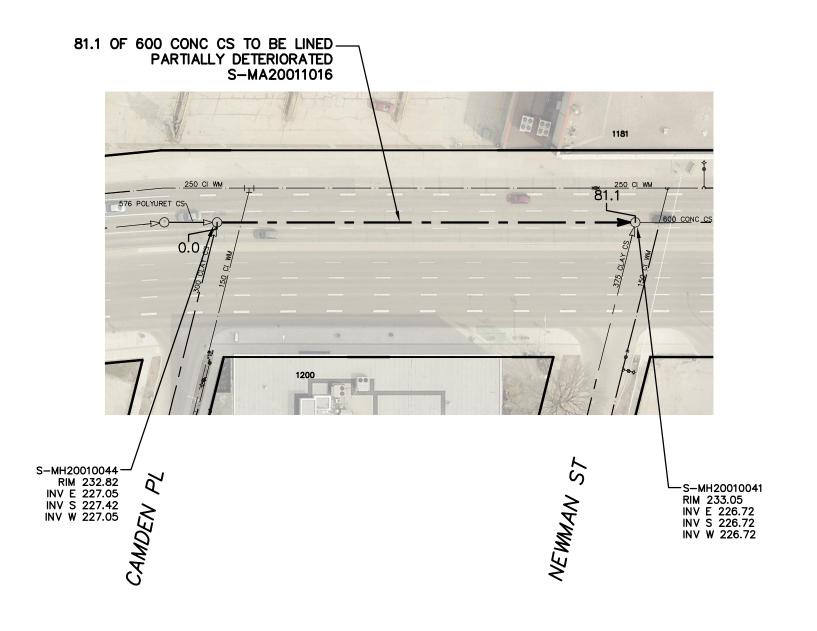
SEWER JUNCTION INFORMATION FROM SEWER VIDEO INSPECTION SEWER ID S-MA20011016 DISTANCE FROM MH ID S-MH20010044 DISTANCE DIAMETER 13.2 150 17.8 150 10 150 45.2 10 45.2 150 75.9 250 10
