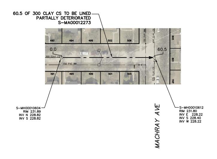
SEWER JUNCTION INFORMATION FROM SEWER VIDEO INSPECTION SEWER ID S-MA00012273 DISTANCE FROM MH ID S-MH00010604 DISTANCE DIAMETER 150 4.4 13.2 150 10 150 21.7 11 21.7 150 27.2 250 27.9 250 10 150 10 41.3 49.0 150 49.7 150 10 52.1 150 54.3 100 10
