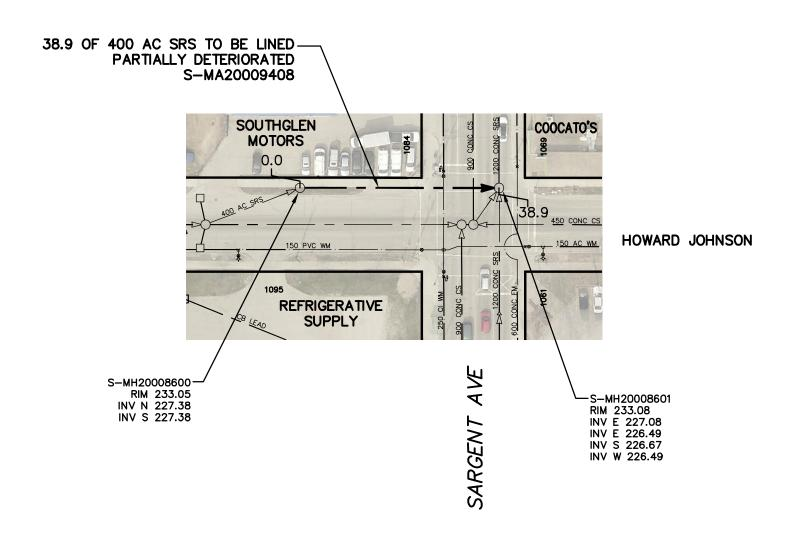
SEWER JUNCTION INFORMATION FROM SEWER VIDEO INSPECTION SEWER ID S-MA20009408 DISTANCE FROM MH ID S-MH2000860 DISTANCE DIAMETER CLOCK NO SERVICE JUNCTIONS
