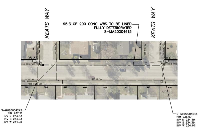
SEWER VIDEO INSPECTION SEWER ID S-MA20004615 DISTANCE FROM MH ID S-MH20004245 DISTANCE DIAMETER 13.7 150 10 27.0 150 9 43.7 150 10 58.4 150 10 72.0 150 10 78.2 150 11
