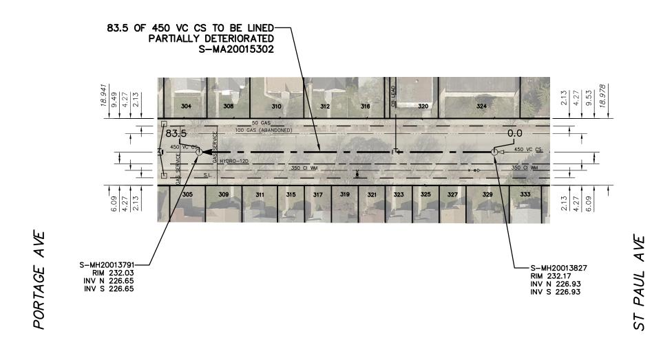
SEWER JUNCTION INFORMATION FROM SEWER VIDEO INSPECTION SEWER ID S-MA20015302 DISTANCE FROM MH ID S-MH20013827 DISTANCE DIAMETER 150 0.8 12 6.3 150 11 14.3 150 11 14.9 150 21.7 150 11 22.4 150 150 30.1 11 30.6 150 37.6 150 150 38.2 12 45.0 150 11 53.0 150 11 53.0 150 58.3 150 12 150 150 59.5 11 68.0 11 76.4 150 81.7 150 11
