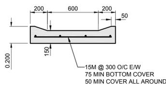
SECTION-B THRU SPILLWAY
