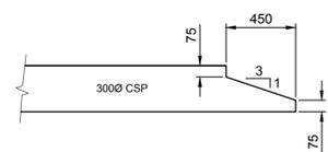
CSP BEVELLED END SECTION
