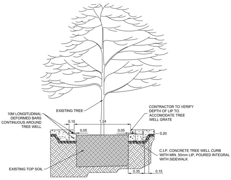
TYPICAL TREE WELL AT EXISTING TREE - SECTION VIEW
