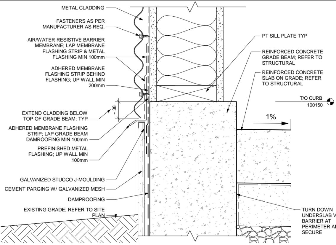
1 SECTION DETAIL - BASE OF WALL - METAL CLADDING
