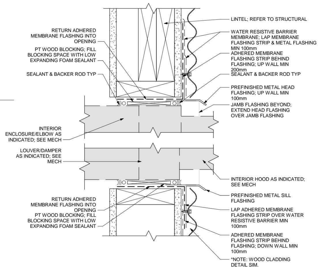
3 SECTION DETAIL - TYPICAL MECHANICAL PENETRATION
