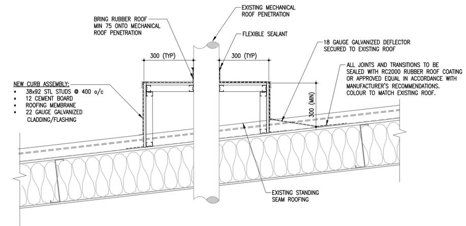
**B** NEW CURB AT TYPICAL ROOF PENETRATION
