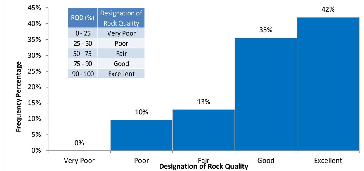
Figure 6-1: Histogram Distribution of RQD within Test holes
