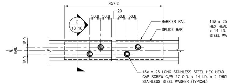
**SPlice BAR TO BARRIER RAIL ASSEMBLY DETAIL**
