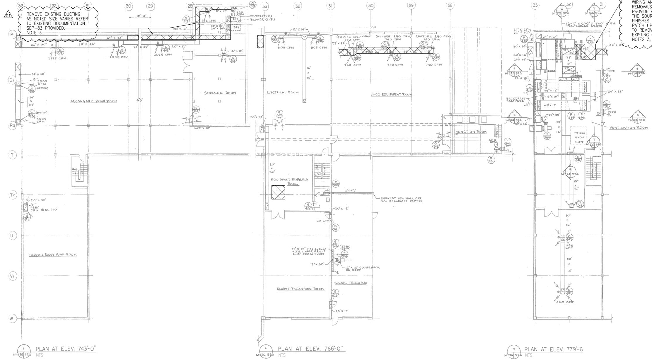
REMOVE EXISTING AHU-688 COMPLETE WITH ASSOCIATED DUCTWORK, PIPING, ELECTRICAL WIRING AND CONTROLS. ALL ASSOCIATED REMOVALS SHALL EXTEND TO THE SOURCES. PROVIDE ALL CAP OFF AND TERMINATION AT THE SOURCES, COMPLETE WITH ALL FINISHES TO MATCH EXISTING CONDITION. PATCH UP ALL REMAINING OPENINGS DUE TO REMOVALS AND REPAIR TO MATCH EXISTING CONDITION. NOTES 3, 4 AND 5.
