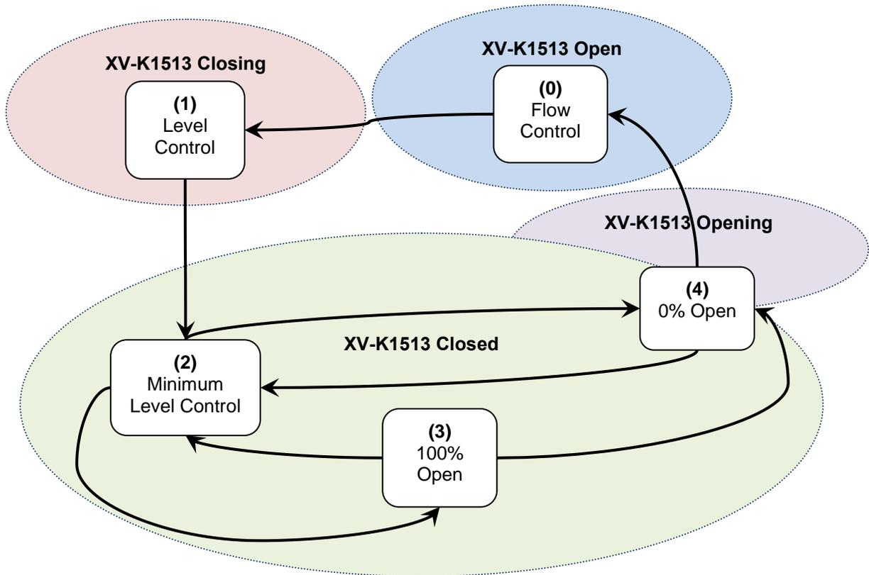
**Figure 3.2-2 YC-K1511\_State - FV-K1511 HRC Effluent to Outfall Weir Gate Possible Request States**
