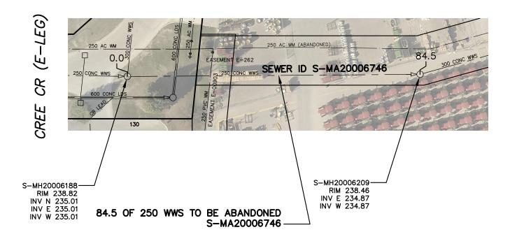
SEWER JUNCTION INFORMATION FROM SEWER VIDEO INSPECTION SEWER ID S-MA20006746 DISTANCE FROM MH ID S-MH20006188 DISTANCE DIAMETER CLOCK 150 4.4
