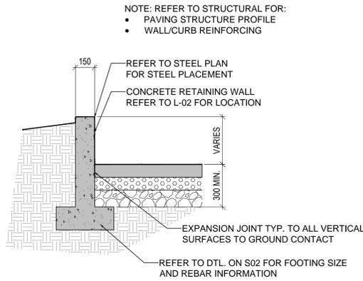
**4** CONCRETE CURB / RETAINING WALL
