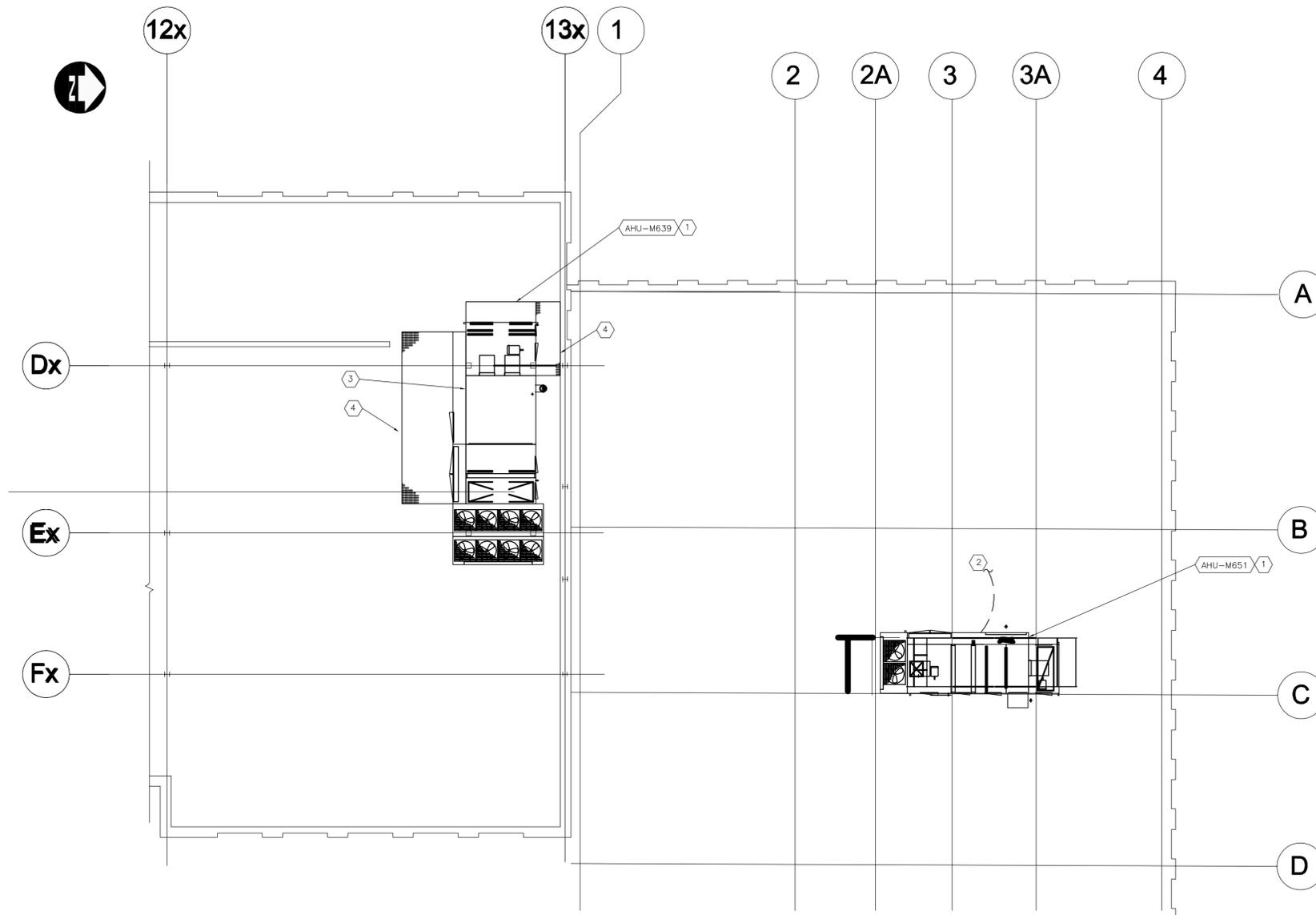
NEW HVAC - PART ROOF PLAN
