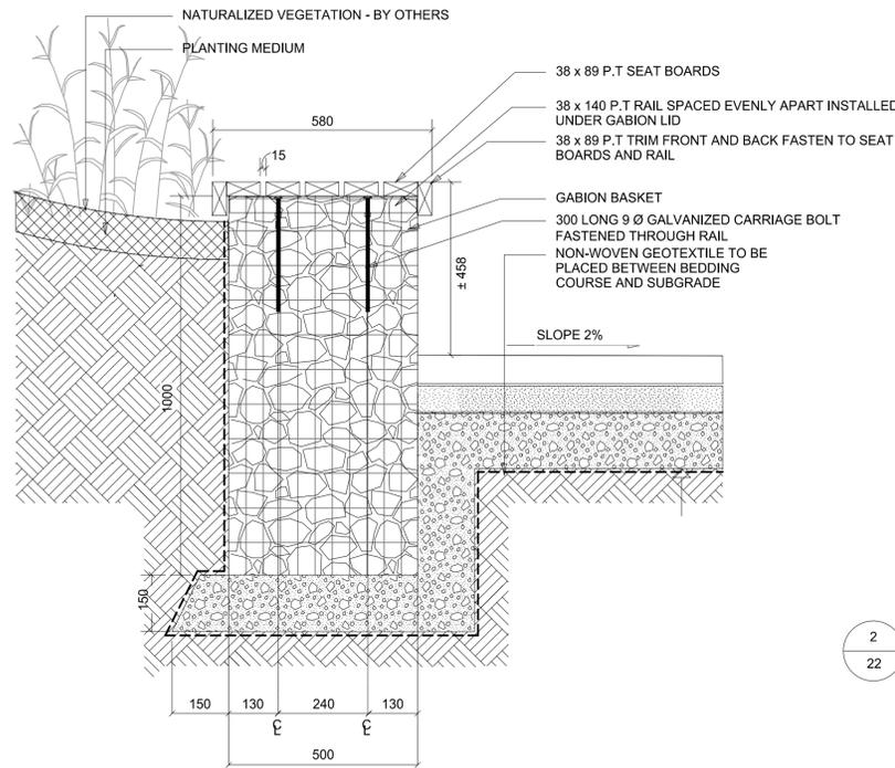
1 GABION SEATWALL SECTION
