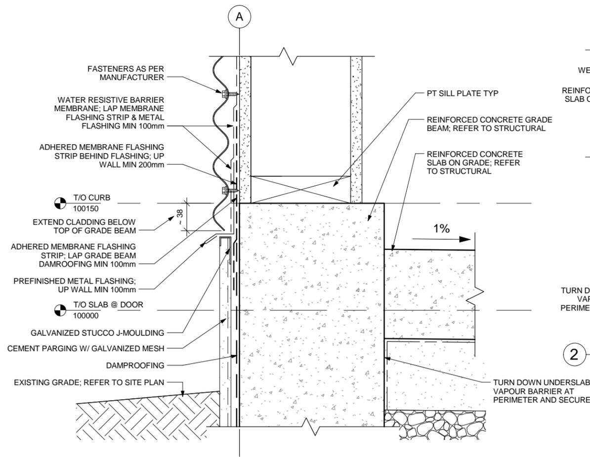
5 SECTION DETAIL - TYPICAL BASE OF WALL
