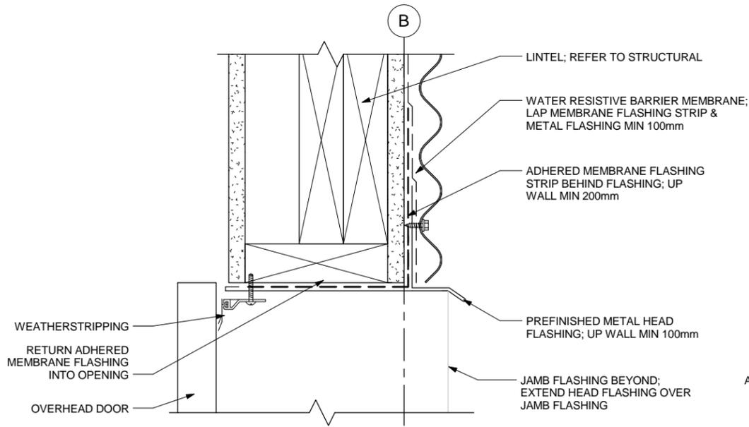
6 SECTION DETAIL - OVERHEAD DOOR HEAD
