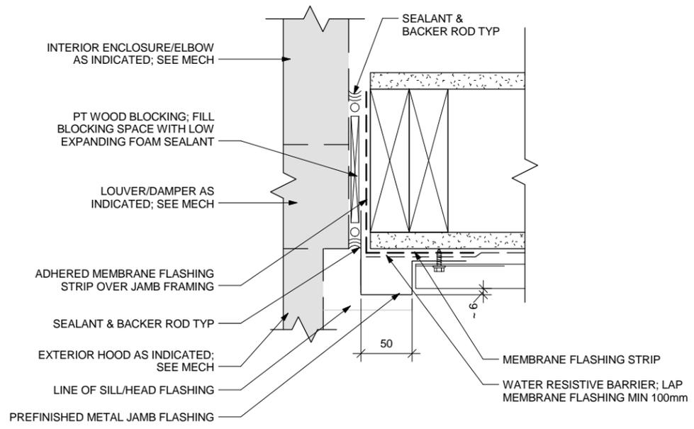
**3 PLAN DETAIL - TYPICAL MECHANICAL PENETRATION**
