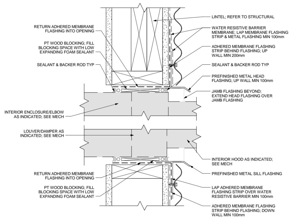
**2 SECTION DETAIL - TYPICAL MECHANICAL PENETRATION**
