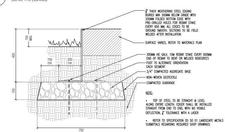
RETAINING STEEL EDGER, TYP.
